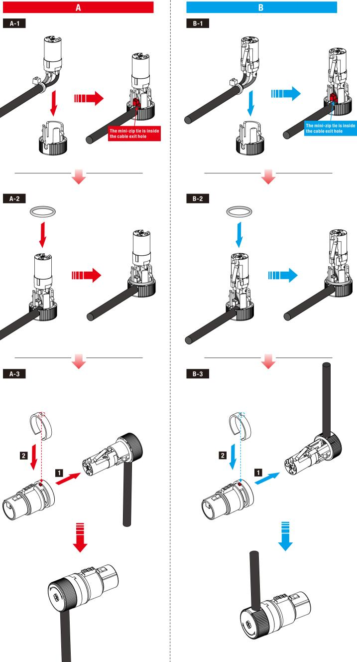
**STEP 6** Depending on your usage needs, as shown below, you can turn the back cover within 100° to align the cable exit to your preferred position.
