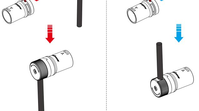
**STEP 6** Depending on your usage needs, as shown below, you can turn the back cover within 100° to align the cable exit to your preferred position.
